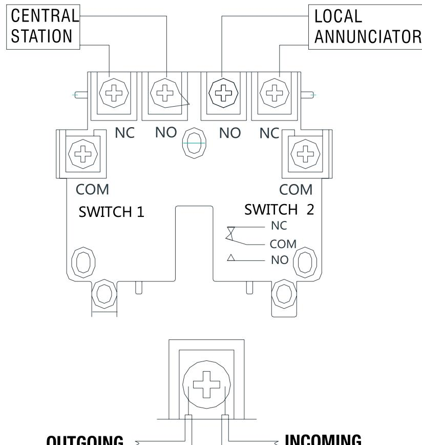
An uninsulated section of a single conductor should not be looped around the terminal and serve as two separate connections
