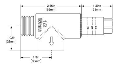
\* Note: Valve showing in the fully open position. Model LV-1 is factory set a approximately 185 psi
