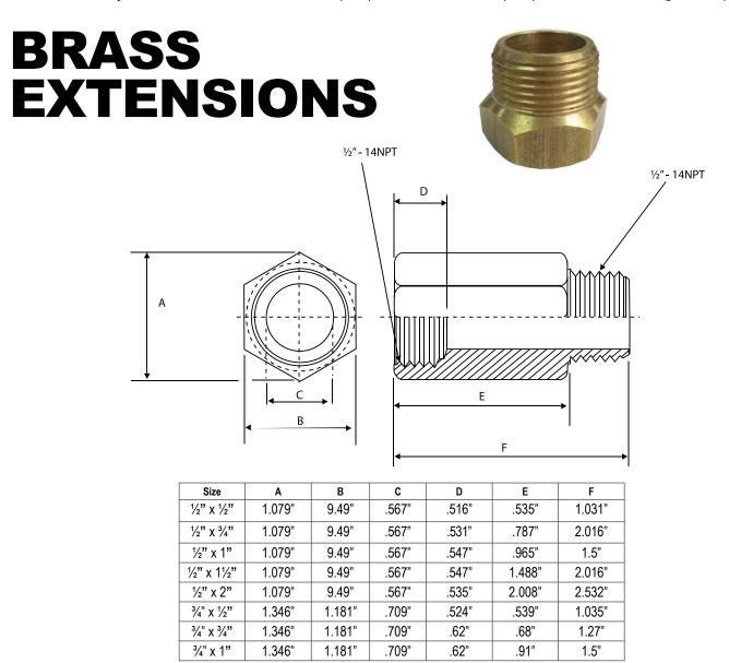
**Caution**: Do not exceed 15 foot pounds torque. Over tightening will cause the sprinkler extension to crack and leak. See additional warnings regarding waiver of lability ands use.
