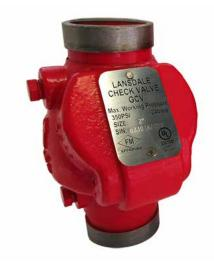
**Note:** Lansdale Check Valves may be damaged by excessively turbulent water flow. They should be installed a reasonable distance from pipe transitions, such as pumps, elbows, expanders, reducers, or similar devices. Typical piping practices suggest a minimum distance of five times the pipe diameter for general use.
