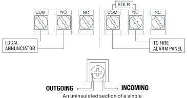
An uninsulated section of a single conductor should not be looped around the terminal and serve as two separate connections
