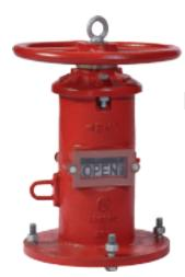
Wall Indicator Post indicates if the valve is in the open or shut position. It is operated by a handwheel and used to operate a valve installed behind a wall. Comes equipped with a 12"O.D. post flange to mount on a wall. Ability to open left or right. UL Listed/FM Approved. Internally and externally red epoxy coated RAL3000 for corrosion protection.
