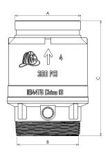
A= 4" (F) NPT B= 4" GROOVED CONNECTION C= 7.875" (200mm)
